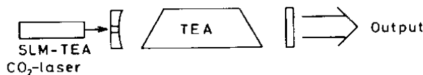
Fig. 4 Injection of an SLM TEA-CO 2 laser pulse into a larger TEA-CO 2 oscillator
